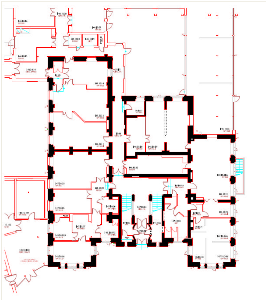
Figure 4. Current CAD plan of the ground floor of the Townsend Building (red and blue) with the original design overlain in black, with dotted lines denoting where original material has been removed. Orientated with north to the left of the image.
