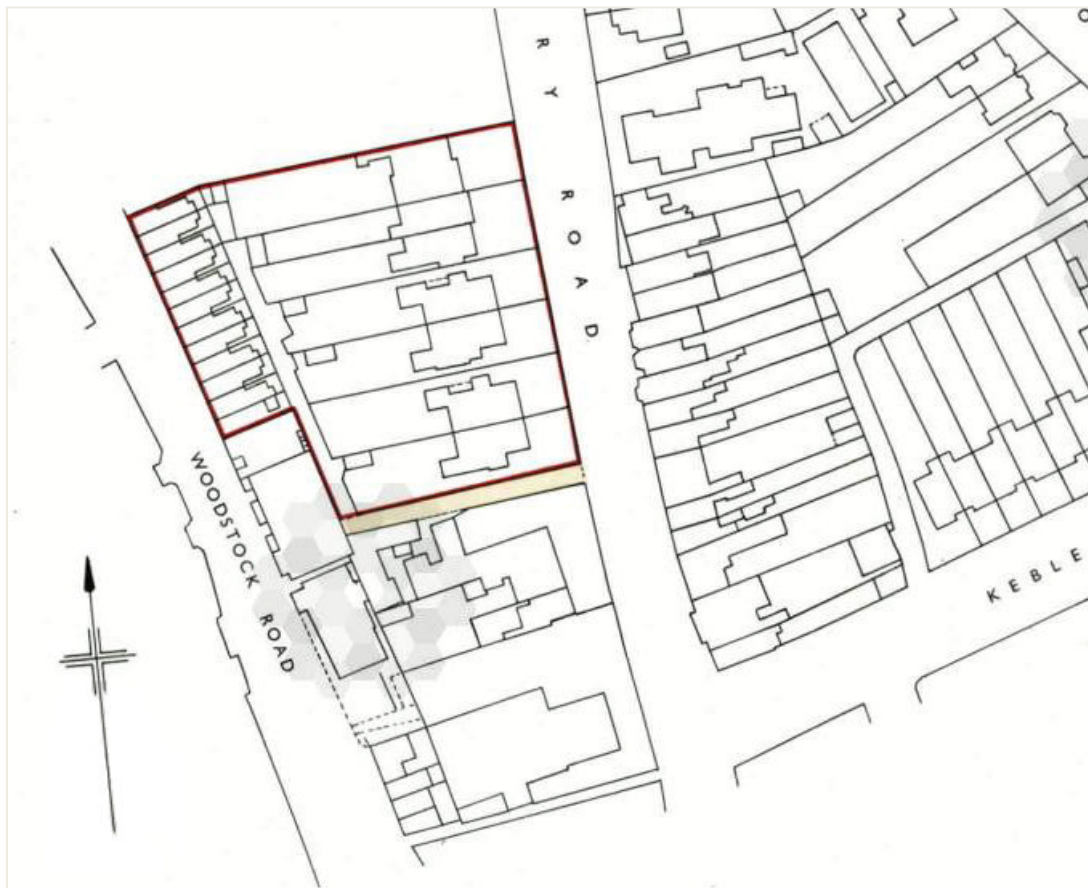
Figure 2. Site plan of 7-19 Banbury Road (outlined in red) from 1969. Note the lack of connecting corridors or extensions (other than the older extension to the north of number 19)
